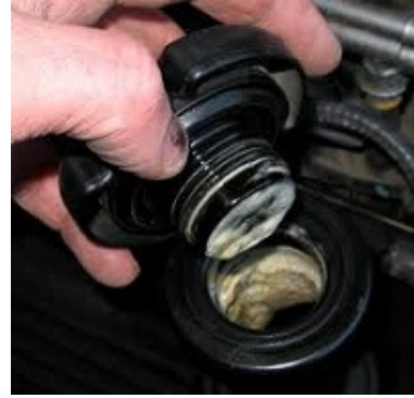
Milky substance under oil filler cap indicating probable engine troubles
