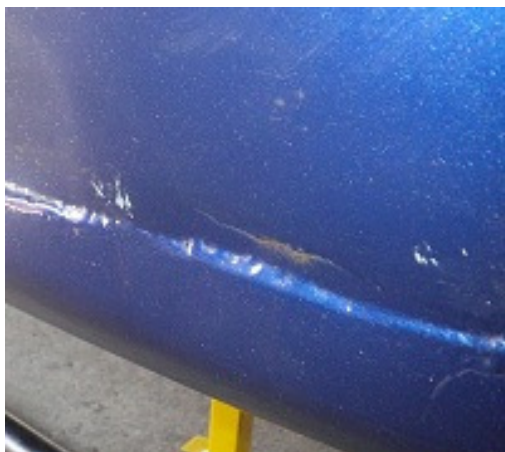
Evidence of a (poor) welding repair adjacent to a bogged up area. This car has had sill damage.
