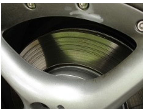
Heavily scored brake rotor. The rotors & pads will need replacing.
