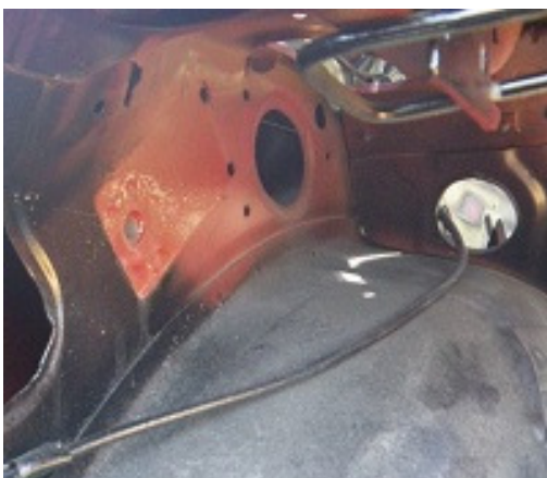
Evidence of a re-sprayed panel. The outside colour is green and the inside is red.
