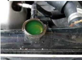
Constant bubbles from the header tank and/or pushing out water may indicate a blown head gasket.
